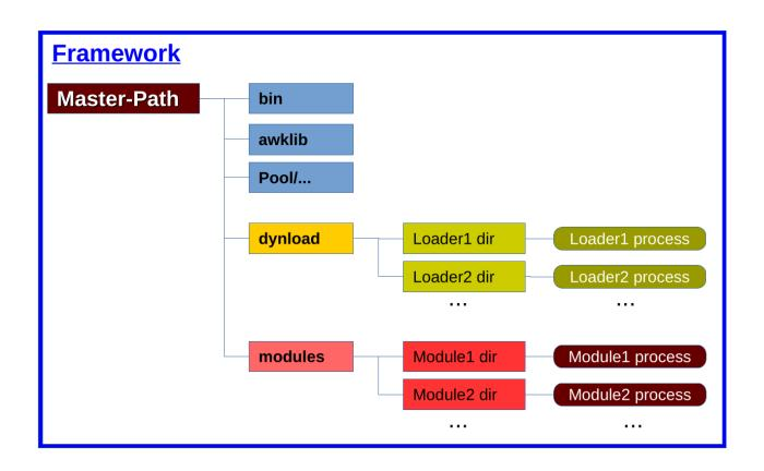
Seen from a loader or module process the Master-Path is always 2 levels up; i.e.: ../../
