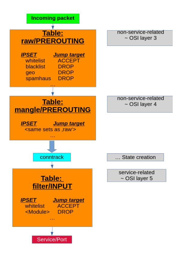
This strictly separates attacks on the NIC (e.g. flood-pings and illegal/unmanaged ports) from attacks on services and avoids that the counters in 'filter' are not pushed-up erratically and reflect the legal access to the services at the 'application layer' (~OSI 5)
