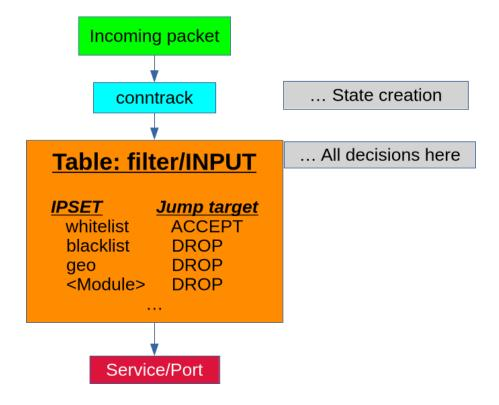
**Watcher 1.5** now blocks packets that are 'not\_service\_related' at 'raw/mangle; PREROUTING' stage which is ~OSI level 3; i.e., simply by their IP address without taking care of protocol and/or service port. This means illegal protocols and or service ports are strictly getting a DROP before reaching the 'filter' stage.
